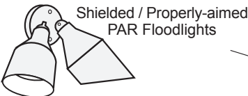
Shielded floodlight that is angled correctly
